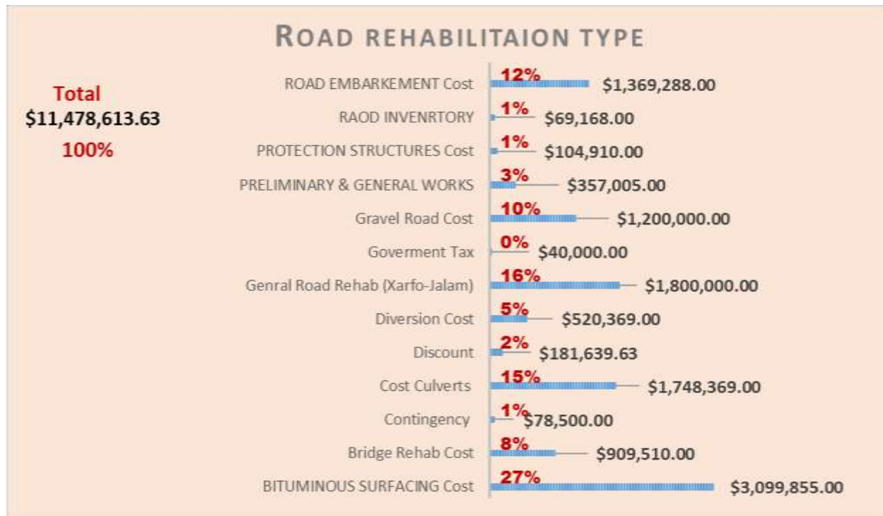
Figure 2. 2: Road Rehabilitation Types
